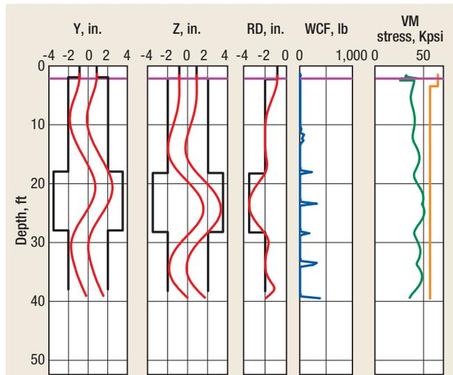
**Fig. 3.** The final output graphs for 0.203 in.-wall coiled tubing shows tubular buckling in the wellbore, maximum radial displacement (RD), wall contact force (WCF) and Von Mises (VM) stress compared to the de-rated allowable yield stress.
