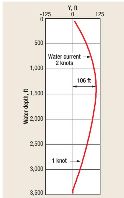
**Fig. 6.** When the slickline is held at surface with 1,076 lb of tension, the maximum lateral displacement from water currents is 106 ft.
