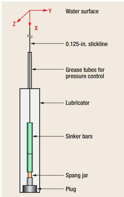
**Fig. 5.** The FEA model simulated a subsea, slickline-jarring, well intervention with 0.125-in. slickline from a vessel in 3,500-ft water depth.
