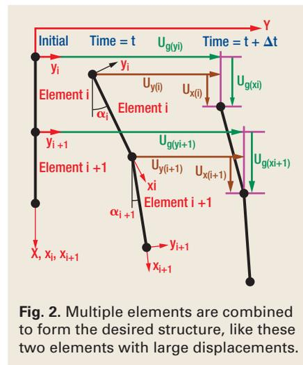
Fig. 2. Multiple elements are combined to form the desired structure, like these two elements with large displacements.
